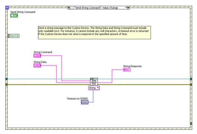
To view an example of the dynamic event pipe, navigate to the <LabVIEW>\examples\NI VeriStand\Custom Devices\Communication Example\ directory and open Communication Example Custom Device Project.lvproj.
