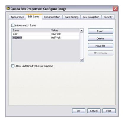
Modify the main page so the operator can set the range of the device.
