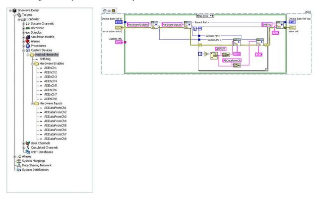
The channels have been organized into *Hardware Enables* and *Hardware Inputs* sections. This device is well-organized and fairly intuitive.
