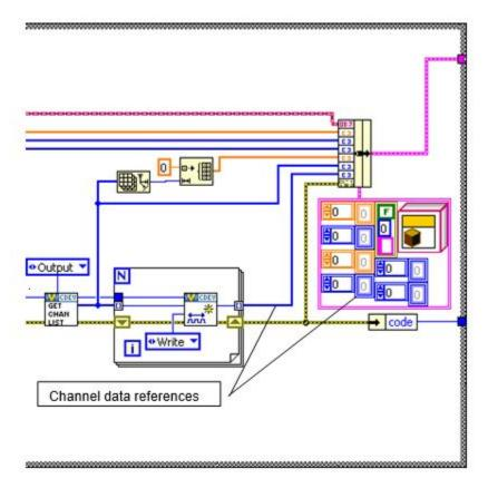
Instead of output channel references, modify the state data cluster to obtain block references to the output channels.
