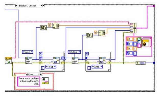
Add the input and output channel references to the state data cluster.
