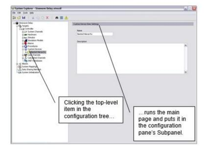
If the developer did not assign a custom page to a new section or channel, the default section or channel page is shown when the operator clicks on the item in the configuration tree.
