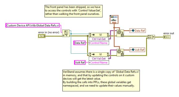
This code can be called only once from within the target custom device. For an inline custom device, it must also be called in the RT Driver **Read Data from HW** case for engine initialization.
