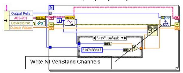
For flat hierarchies, the reference array corresponds one-to-one with channels. This is because they were created on the host computer. The first channel created is the 0th element of the array.
