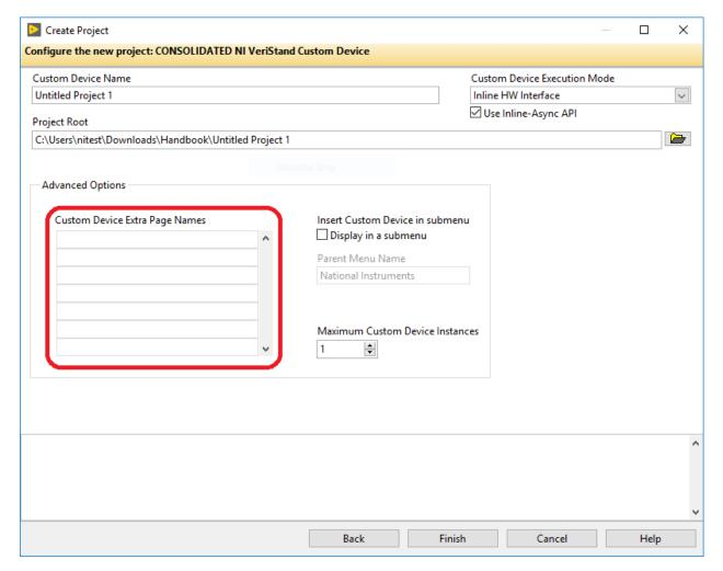
The *niveristand-custom-device-wizard* generates the page, GUID, and XML Declaration. The wizard then includes the page in the build specification. You will find the extra page template in the *Page Template.vit*. This file is located at Custom Device API.lvlib\Templates\Subpanel Page VI.
