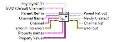
The device or device subsection is specified by *Parrent Ref in*. If the *Channel Name* you specify already exists, the VI overwrites the existing channel settings without affecting any custom properties. The VI can be called from any VI that runs on the host computer.
