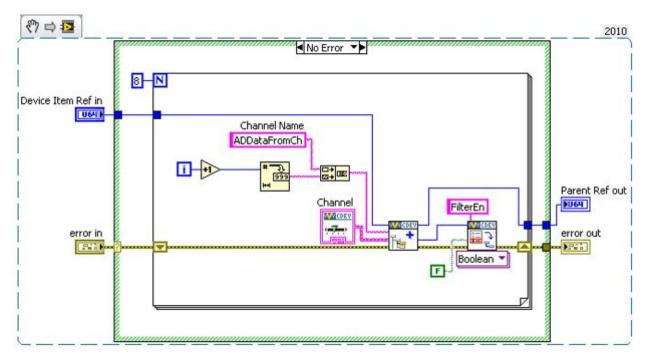
Replace the string constant with a global variable that has the same default value as the constant. Use the global variable *Constants.vi* by navigating to **Custom Device Name> Shared.lvlib** » **Shared**.
