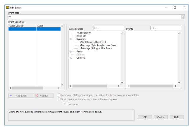
The two message events activate when *NI VeriStand – Send Custom Device Message.vi* is called. The following Lab-VIEW code displays how to send information to VeriStand's Dynamic Message Events.
