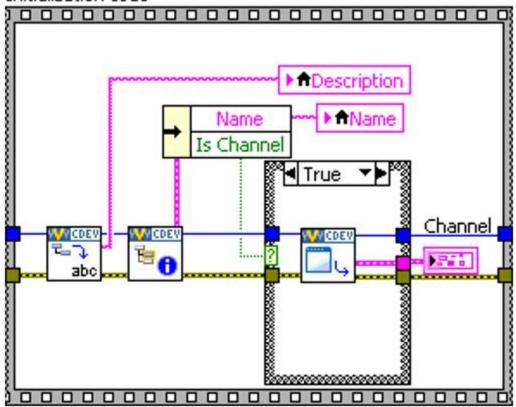
You should use the Boolean outputs from functions in the API to make sure that you are operating on a valid reference. In this case, we will only retrieve the channel data if we have a valid channel reference.
