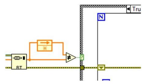
Simple change detection can fail due to floating point precision issues. Change detection with tolerance avoids these precision issues. You should use tolerances that avoid false triggers.
