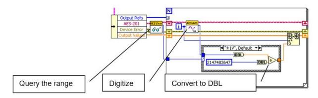
Send the channel data to the rest of the VeriStand system by writing to the Output Reference.
