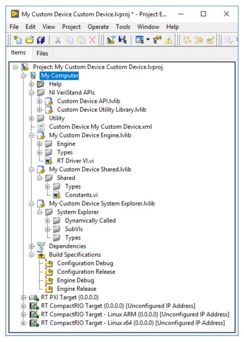
The Custom Device API library and Custom Device Utility Library contain most of the type definitions, template VIs and LabVIEW API needed to interact with VeriStand data and timing resources. They allow the VI to behave as a native task in the VeriStand Engine.
