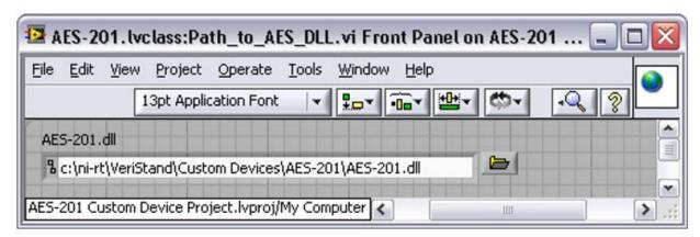
For ease of maintenance, deploy the .so file to C:\ni-rt\VeriStand\Custom Devices\<Custom Device Name>\library>.so.
