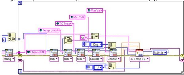
There are several advantages to this architecture. The operator is free to add, remove, and reorder channels. Only the desired channels are configured. This makes writing data to the custom device FIFO efficient.
