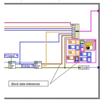
The original version of the custom device automatically creates an index of each channel data reference.
