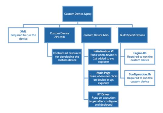
The XML file tells VeriStand how to load, display, use and deploy the device. The VI Libraries define the behavior of the device. One library is for configuration and the other is for the engine.
