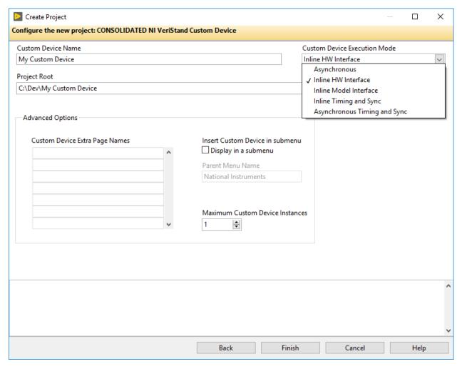
The selected mode determines when the device will run with respect to the other operations performed by the VeriStand Engine. There are five device frameworks available. Three of the frameworks are for custom devices, and the other two are for custom timing and synchronization devices.
