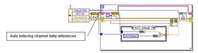
You should modify this code to write the block reference. In the following example, the channel block data references are written together outside the loop rather than channel-by-channel within the loop.
