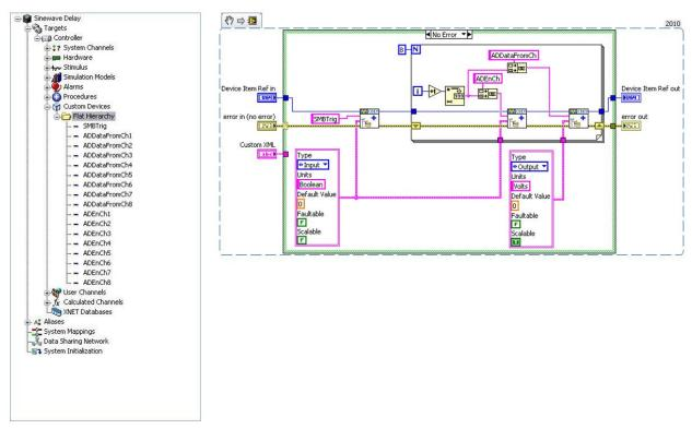
In this example, all of the channels are under the main section in the configuration tree. While it is easy for the operator to determine how many channels are available, the type of channel is unknown. Also, the channel function is only implied by the name.
