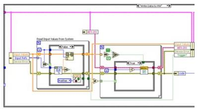
The triggering VI is useful in asynchronous custom devices that do not execute in line with the primary control loop (PCL). An asynchronous device might iterate multiple times in a single iteration of the PCL. This triggering VI will only assert on the desired edge of the transition.
