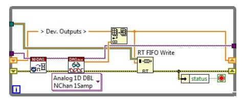
The hardware data returns from the DAQmx driver in the same order as the channel references in the asynchronous custom device FIFO.
