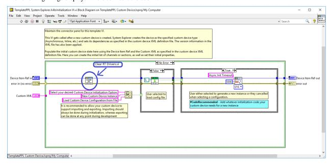
Inside the Action on Compile VI, add a *Set RT Driver* subVI to re-insert the corresponding RT Driver paths before system deployment. VeriStand keeps a copy of the deployed system definition in the local cache unless the system definition is unmodified between deployments. The latest changes are preserved, allowing VeriStand to use the "complete" system definition from the local cache during deployment.
