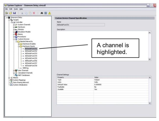
The default pages allow the operator to set a description for the section or page. VeriStand retains this data in the System Definition (.nivssdf) file.
