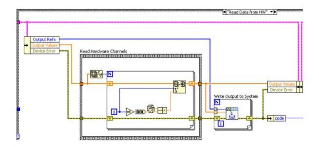
Replace the Read Hardware Channels frame with the API call to digitize. Convert the 32-bit raw data to DBL data, depending on the range of the AES-201.
