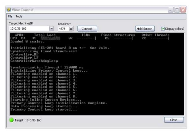
Check the console for messages to determine if the non-default configuration is active. You should also map the ADDataFromCh < 1..8 > channels to a simple graph to ensure they display the expected signals.
